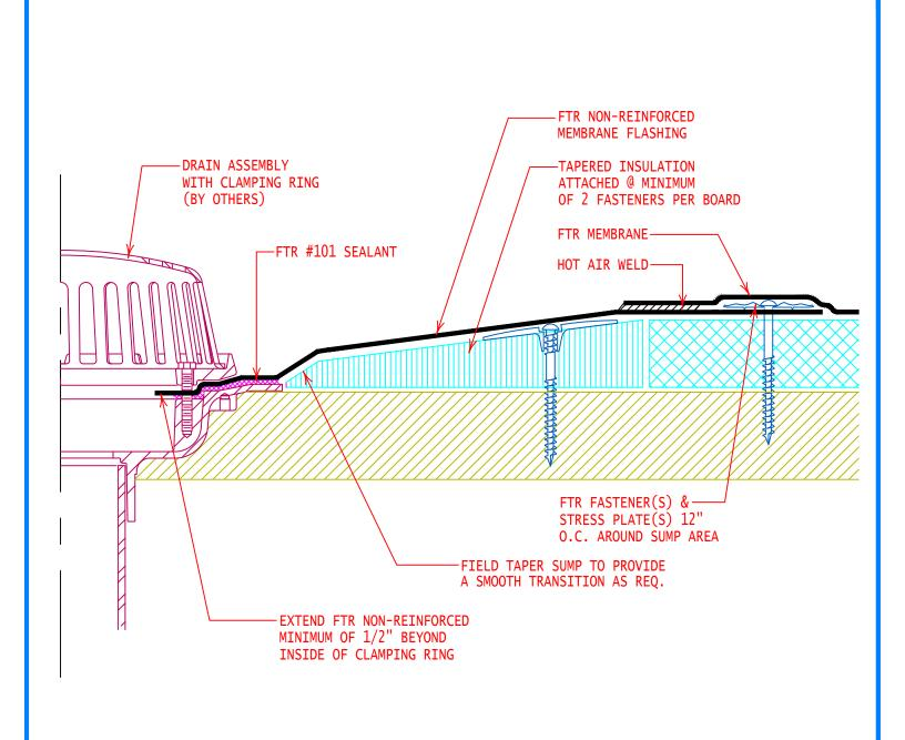
NOTE: USE TAPERED ROOF INSULATION (EDGE STRIPS) TO CREATE DRAIN SUMP. IF TOTAL INSULATION THICKNESS IS LESS THAN OR EQUAL TO 1 1/2 IN., TAPER 12 IN. FROM THE DRAIN CENTER. IF TOTAL INSULATION THICKNESS IS GREATER THAN 1 1/2 IN., TAPER 18 IN. FROM DRAIN CENTER.
